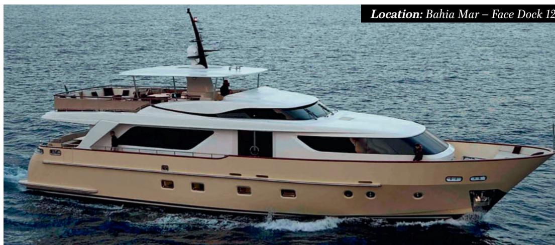
LOA: 90'6" BEAM: 23'5" DRAFT: 5'3" ENGINES: 2 x MAN V12 FUEL CAPACITY: 4,228 GAL. WATER: 660 GAL. MAXIMUM SPEED: 17 KNOTS CONSTRUCTION: COMPOSITE RANGE@11 KNOTS: 2,000 NM
